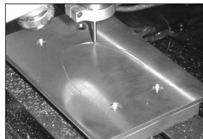
Figure 9. Computer-generated Orthos archwire production. Consistent use of the same ideal arch form throughout treatment aids in early arch-form integrity.
